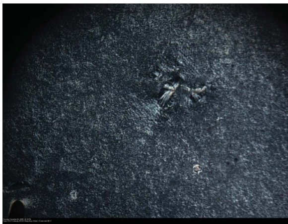
Figure 7. Representative PLM images ( 250\times magnification) of thermotropic LC phases of gemini imidazolium salts with n -hexyl spacers: (a) n -dodecyl tails ( 8a ) at 100^\circ\text{C} ; and (b) n -tetradecyl tails ( 9b ) at 110^\circ\text{C} .
